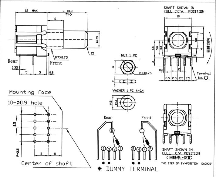
NOTE: 1. TOLERANCES UNLESS OTHERWISE SPECIFIED: ±0.3mm,angle: ±5\* 2. ACCESSORY PARTS: Ø7 HEXAGON NUT ONE PIECE & WASHER ONE PIECE
